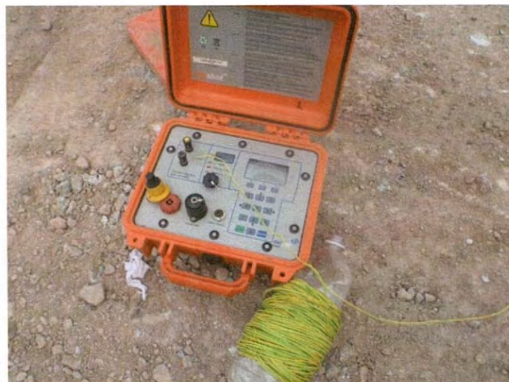
FIGURA 28. Digi shot (blaster) y harness.
